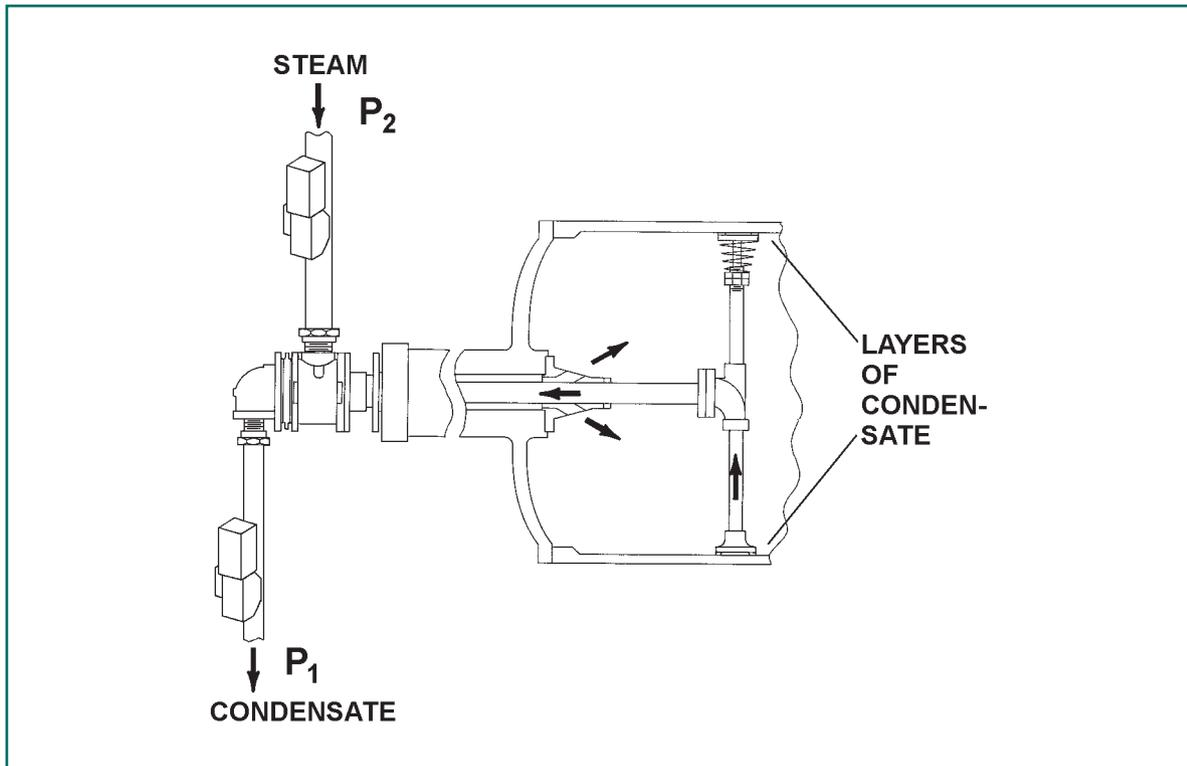
Figure 1. The dryer siphon assembly, inside of the cylinder, with the supply and inlet piping and the outlet piping.
